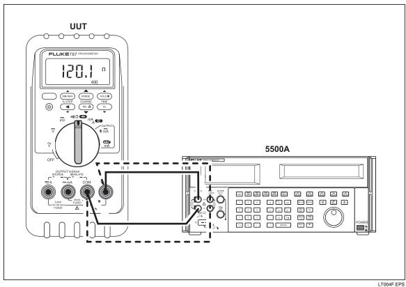
Figure 8. Resistance Measurement Test Connections
