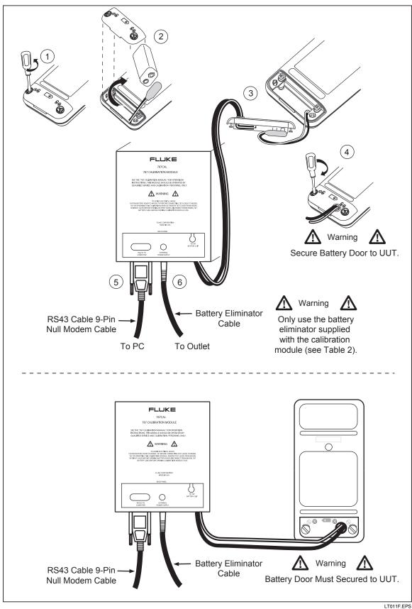
Figure 13. Connecting the 787 Calibration Module to the UUT
