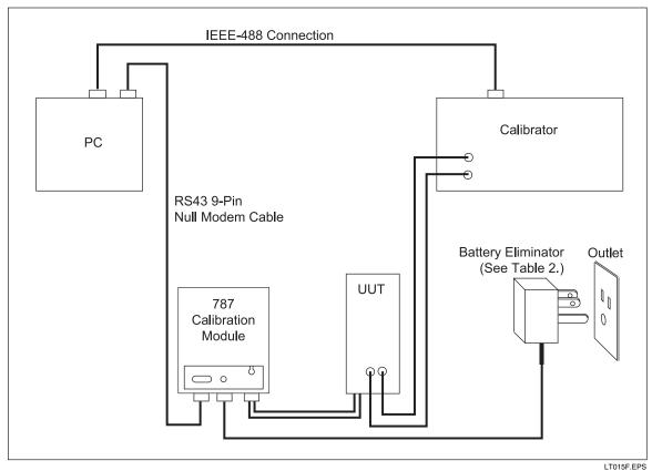
Figure 12. Calibration Connections for the 787 ProcessMeter
