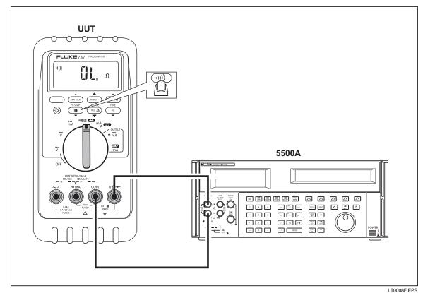
Figure 7. Continuity Test Connections
