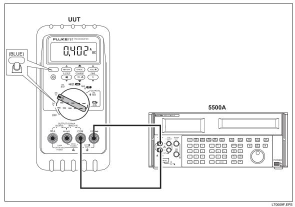
Figure 10. AC/DC Voltage Measurement Test Connections
