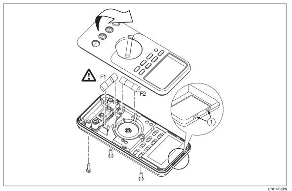
Figure 2. Replacing a Fuse
