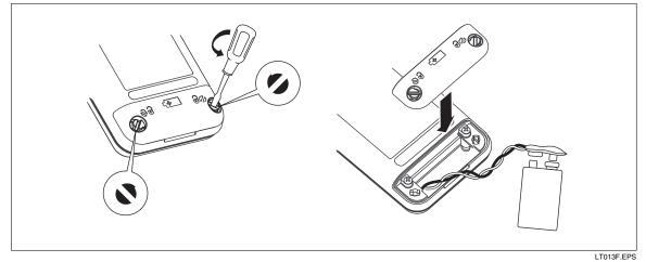
Figure 1. Replacing the Battery
