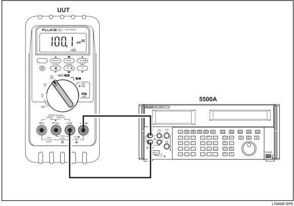
Figure 9. DC mV Measurement Test Connections
