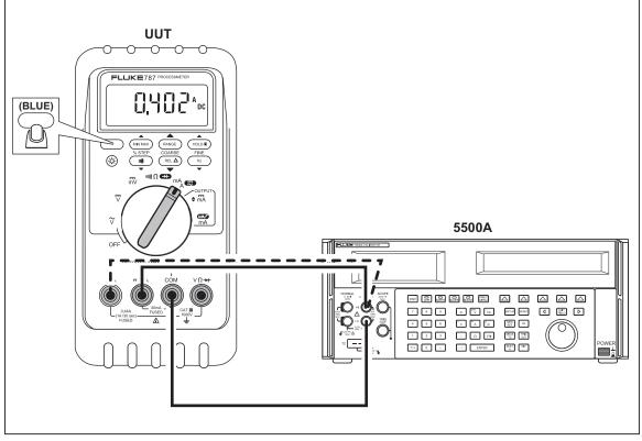
**Figure 5. Current Measurement Test Connections**
