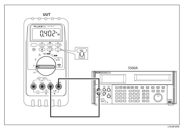
Figure 11. Frequency Measurement Test Connections
