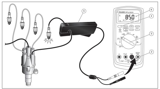
Figure 9. Measuring RPM with Inductive Pickup
