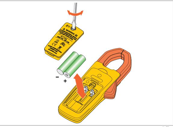
Figure 5. Battery Replacement
