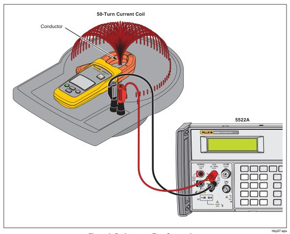
Figure 3. Performance Test Connections
