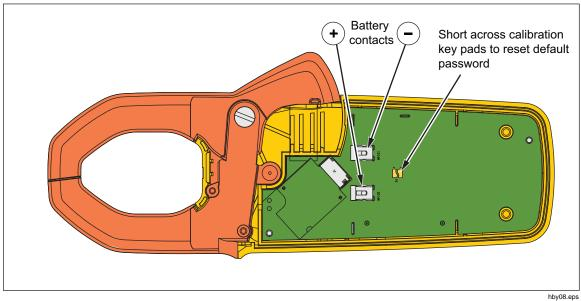
Figure 4. Calibration Password Reset
