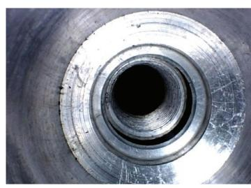
Photo above: Spark plug port inspection
