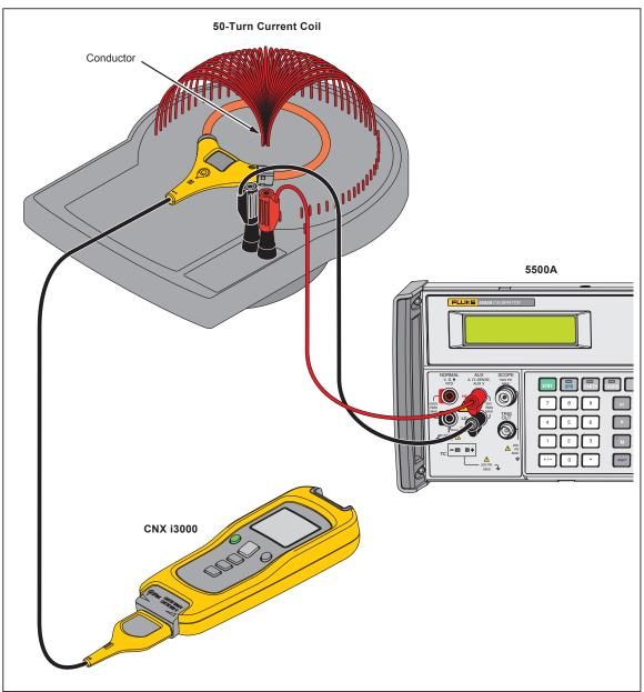
Figure 3. Performance Test Connections for Applied Current
