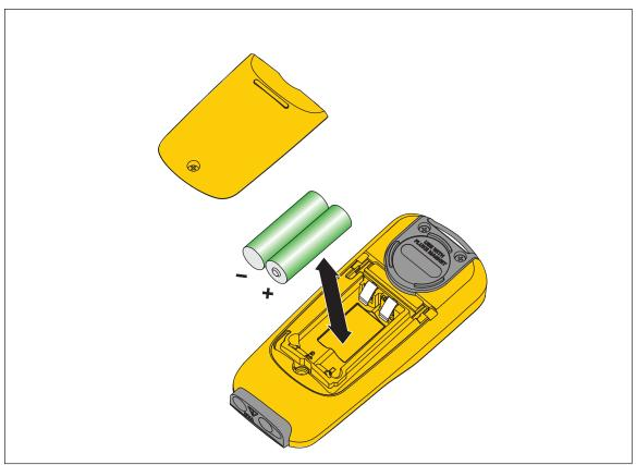
Figure 5. Battery Replacement
