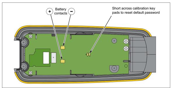
Figure 4. Calibration Password Reset
