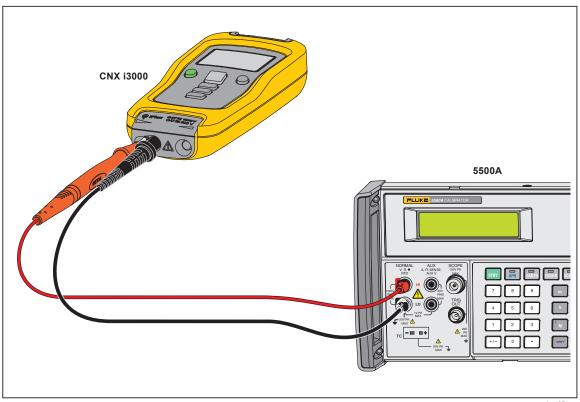
Figure 2. Performance Test Connections for Simulated Voltages
