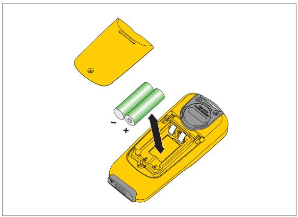
Figure 4. Battery Replacement
