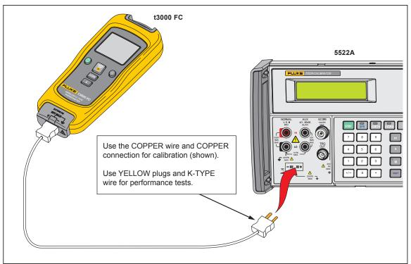
Figure 2. Performance Test and Calibration Connections
