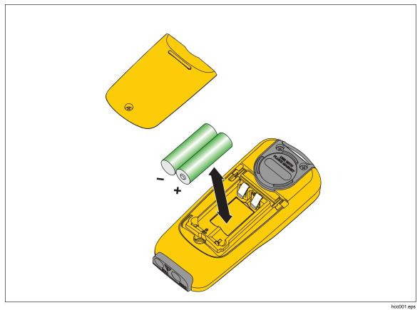
Figure 4. Battery Replacement
