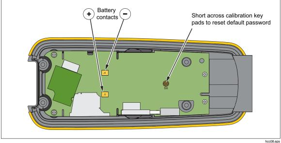
Figure 3. Calibration Password Reset
